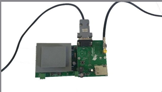
TOP VIEW OF THE RMU WITH ITS BATTERY SUPPLY
